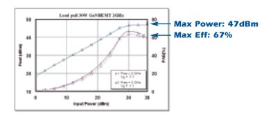
Example of simulated results using Auriga Model compared to the measured data of a 50W GaN HEMT device
